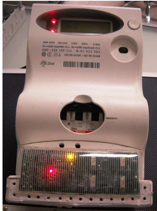
**Example of installation of Ekovar directly on electronic meter of electricity**
