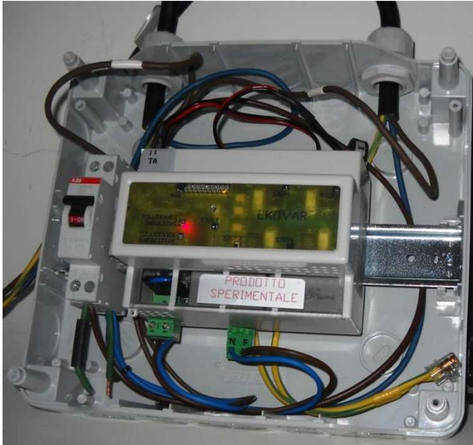
**Example of installation of Ekovar in switchboard modular DIN rail support.**
