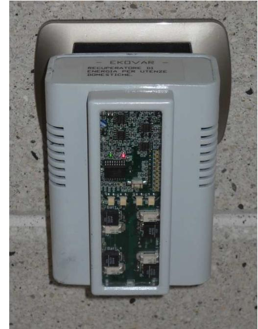
**Example of installation of Ekovar plugged into an outlet of electricity for domestic use**
