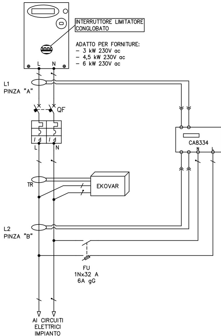
APPARATO DI MISURA E ANALISI RETI ELETTRICHE
